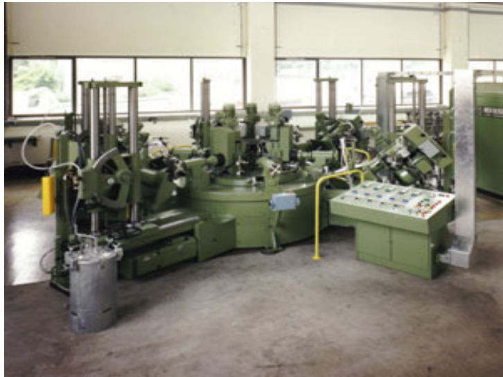
Figure 2 Example of 6 station rotary configuration for assembly
